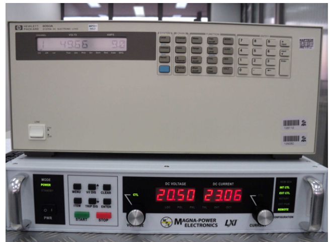
Fig. 10. Front panels of the fuel cell emulator Magna Power Electronics and the programmable electronic load HP 6050A.
